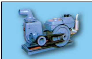
PUMP COUPLED WITH ENGINE * This picture doesn't show belt cover for safety belt cover should be install.
